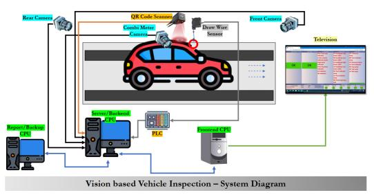
The following steps provide an overview of the end-to-end Vision based Vehicle Inspection solution control flow:
