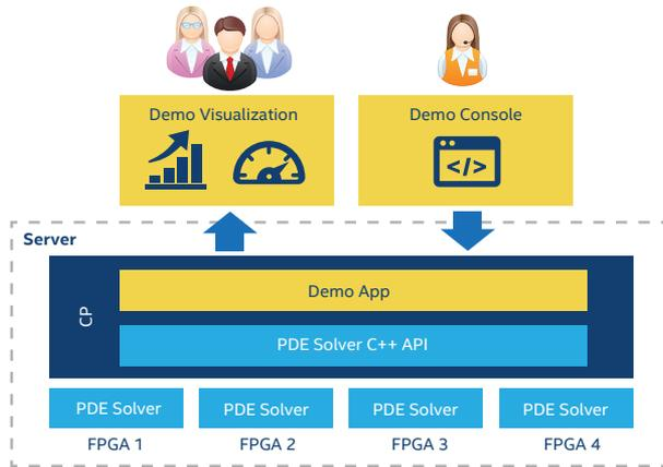
Figure 2. Data Center Orchestration Flow of Acceleration Platform
