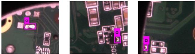
Before boards are manually inspected, the AOI system marks all suspected anomalies and indicates them on a monitor, so visual inspection is streamlined.
